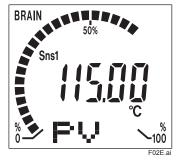
Figure 2. Integral Indicator Display Example.
